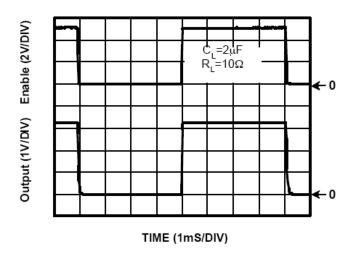
Figure 5. Chip Enable Transient Response
