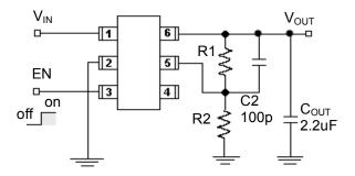
$V_{OUT} = 1.215 (R1+R2)/R2$ C2 is unnecessary when R1 or R2 < 20K PG pin is only available in the SOT-26 package Connected to output for Power Good or left floating
