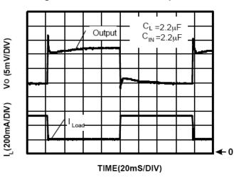
Figure 4. Load Step (1mA~300mA)
