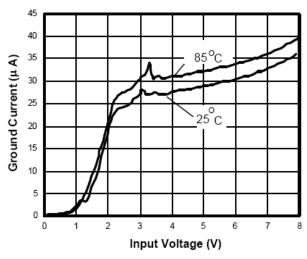
Figure 1. Ground Current vs. Input Voltage
